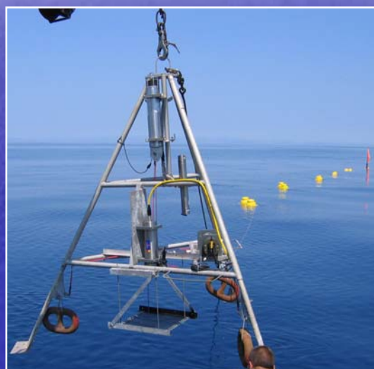
ISIT (Intensified Silicon Intensifier Target); a lander instrument of the type that may be used for bioluminescence monitoring in KM3Net site survey.
