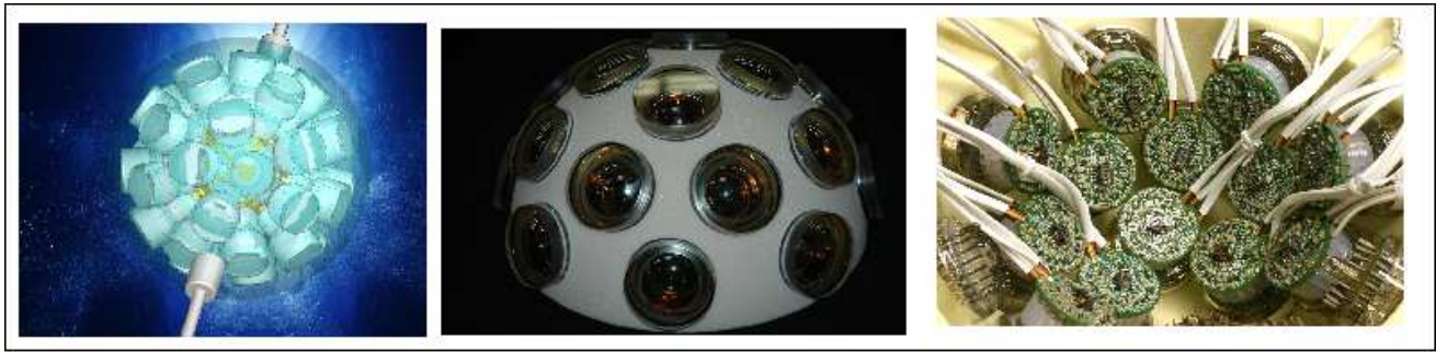
Fig. 5. Technical drawing (left) and first prototype (middle and right) of an OM with several small PMTs (taken from [8]).
