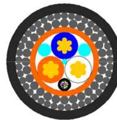
Figure 7-19: Cable option for 3-Phase AC with 3x25 mm 2 conductors.
