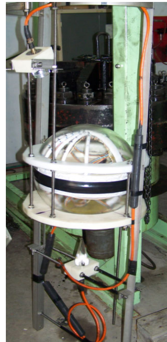
Figure 6-13: LIMS glass housing and mechanics
