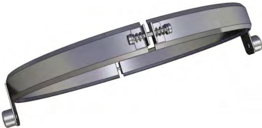
Figure 3-30: The spring loaded titanium connection ring
