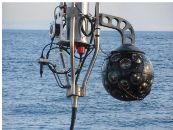
Figure 1: Photograph of the first KM3NeT optical module, just before deployment 40 kilometres off the coast of Toulon, France.
