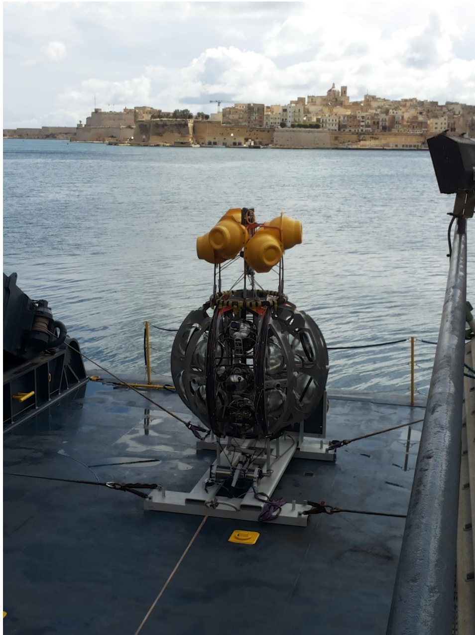
Figure 1: Prototype of a KM3NeT string (mounted on the launcher vehicle) on board the Nautical Tide on its way from Malta to the deep-sea site, 100 kilometres off the coast of Portopalo di Capo Passero, Italy.
