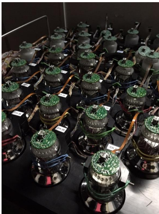
Figure 4: PMTs in the tray before the test.
