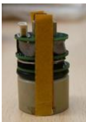
Figure 9: Fully assembled prototypes of the piezo sensors with digital readout.
