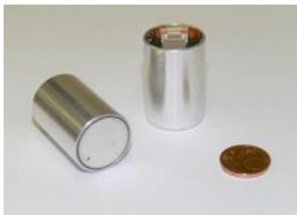
Figure 8: The integrated piezo and electronics before insertion into the aluminum tube.
