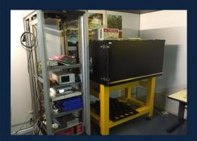
The DarkBox is used to measure the PMT dark rate, equalize gain, determine spurious pulses and timing characteristics such as transit time and transit time spread. A complete calibration takes about 10 hours of which 9 hours are used for PMT conditioning in darkness. 7000 3-inch PMTs have been tested at Naples using the «DarkBox» facility.
