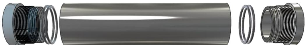
Figure 5: Option 2 for the deep sea casings for the PD boards. This design is preferred for harder stainless steel alloys such as alloy 17-4 and results in a smaller outer diameter.
