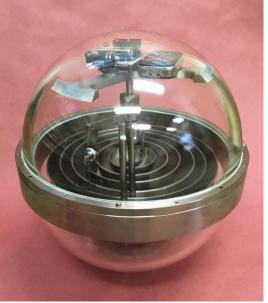
Figure 6: (left) first immersion test of the Bathysphere prototype. (right) final version of the Bathysphere ready for deployment. The glass sphere is identical to those already deployed by KM3NeT.
