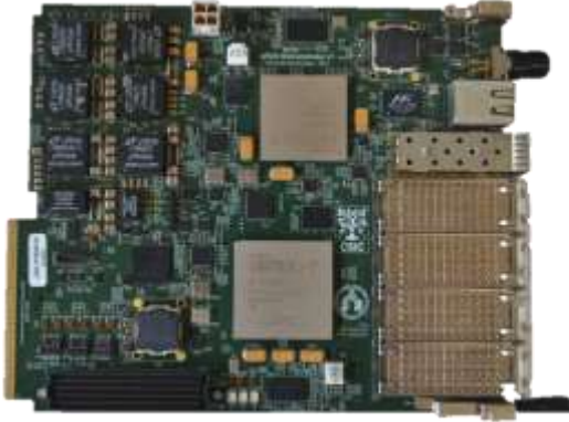
Figure 7: Board where the latency of the transceivers has been tested. It contains a Xilinx Virtex 7 FPGA.
