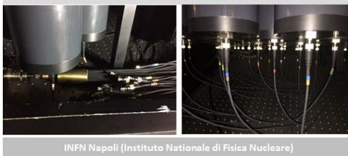
Optical splitter 1 input → 70 outputs
