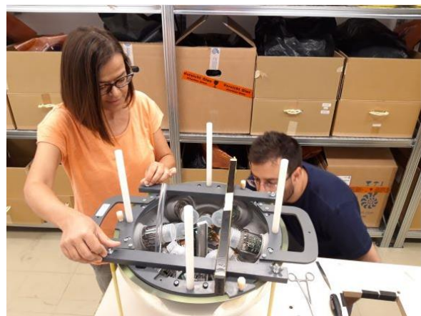
Integration of the dummy DOM in the DOM integration site in Athens
