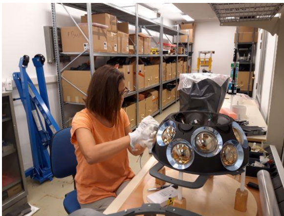
Integration of the dummy DOM in the DOM integration site in Athens
