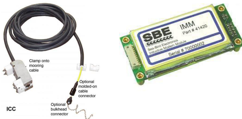
Figure 38: Seabird Inductive Modem Module (RS422 standard).
