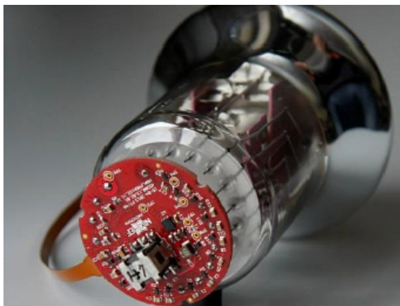
Figure 16: PMT tube with base(left) and PMT base block diagram (right).
