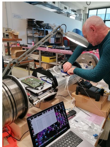
Figure 13: Optical splicing in the JB vessels at Elmacom.
