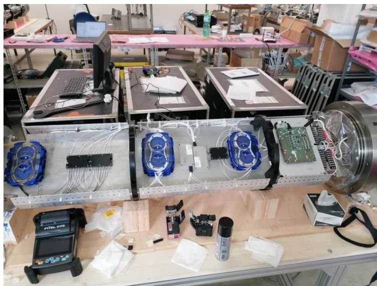
Figure 11: Picture of the fully implemented optical Junction Box vessel.
