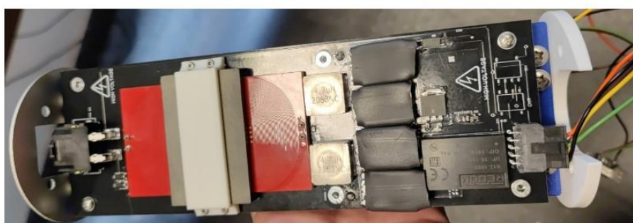
Figure 2: Pictures of the transducer of the acoustic beacon
