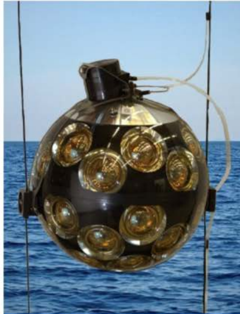
1 optical module = 31 photomultiplier tubes
